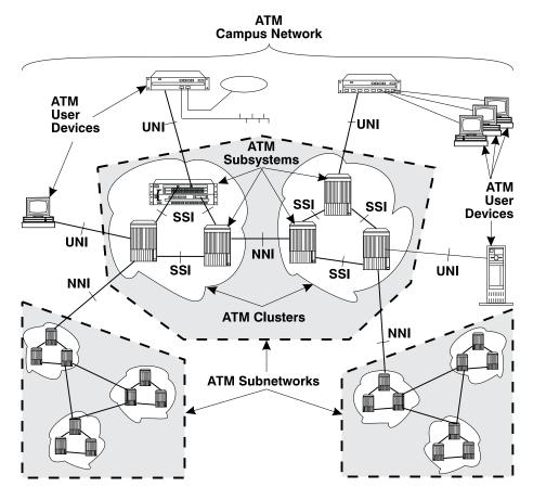
Figure 3-1. Components of an ATM Campus Network
